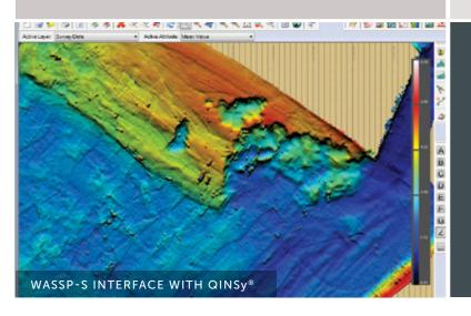
Due to its ease of installation, WASSP Multibeam was used for survey reconaissance of the MV Rena grounded on the Astrolabe Reef in New Zealand. Within 48 hours of equipment delivery surveyors had located multiple submerged containers in depths of up to 80 metres.
