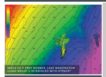
WASSP data is displayed in real-time, enabling you to make on the spot decisions. Instantly locate underwater debris or structures that might pose a hazard, and determine their precise size, shape and position.
